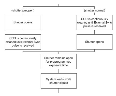
Figure 14. Continuous Cleans Operation Flow Chart
